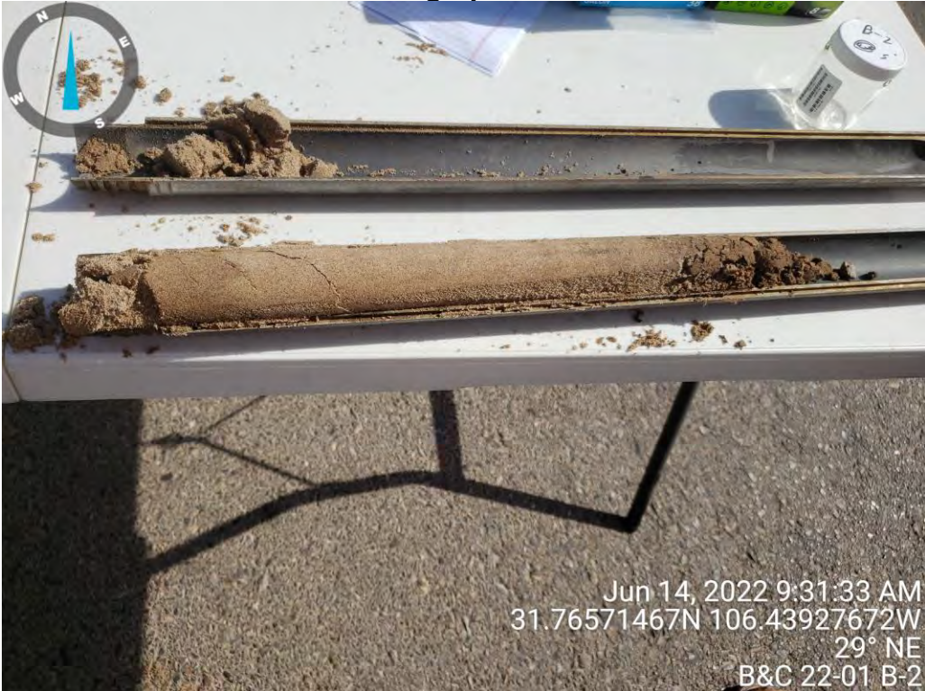
View of split spoon sample at B-2.
