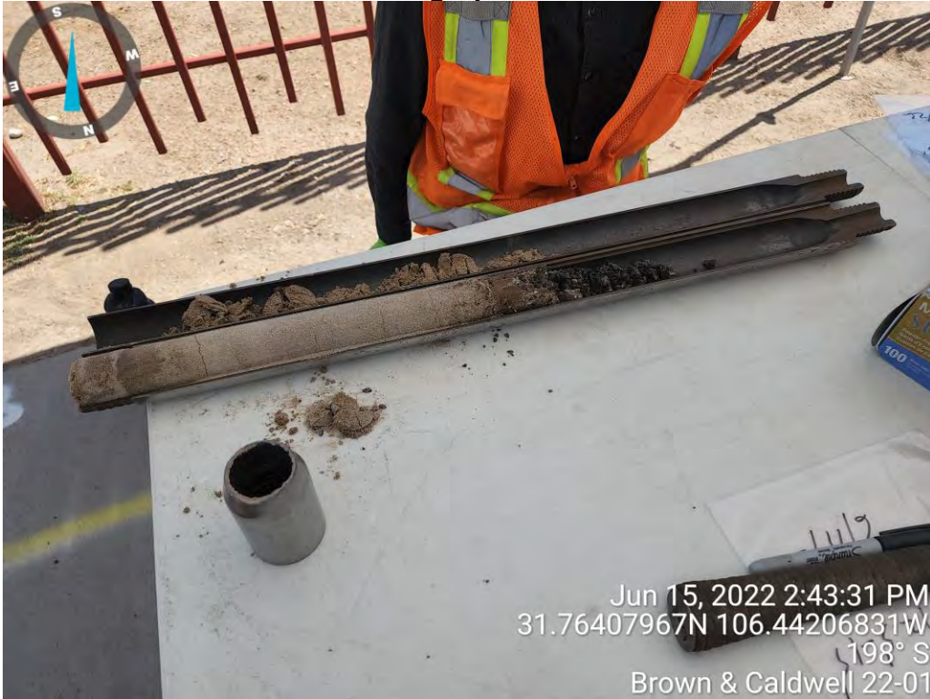
View of asphalt and soil sample on the split spoon observed at B-13.
